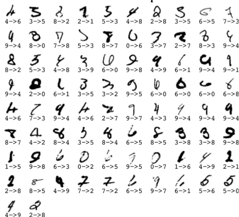
Figure 12.2. Example of digit recognition mistakes by the algorithm in LeCun et al 1988. Below each digit, the image shows the true label and the computer label.
