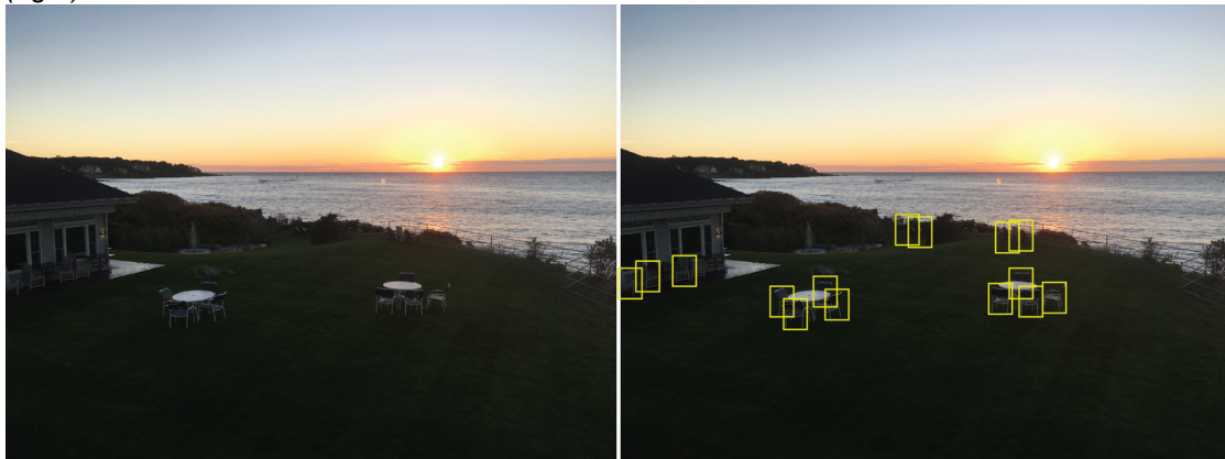
Figure 9.2: Object localization. The task involves taking an image (left) and localization all instances of a given object class (e.g., chairs in this example) by drawing a box around them (right).
