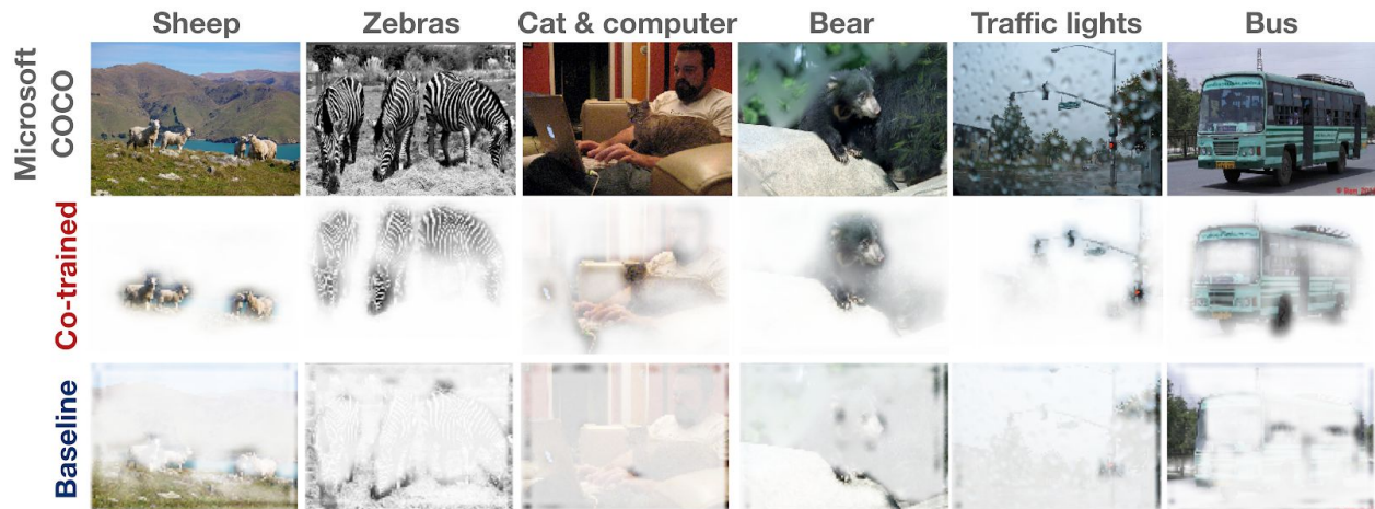
Figure 5. Learning what and where to attend. The top row depicts representative images from the Microsoft COCO dataset depicting object categories also present in ILSVRC12 (which was used for training the system). In the middle row, each of these images is shown with the transparency set to the attention map it yielded in the attention network by Linsley et al [179] trained with human supervision (see text for details). Visible features were attended to by the model, and transparent features were ignored. Animal parts like faces and tails are typically emphasized, whereas vehicle parts like windows and windshields are not. Co-training the attention network with human supervision yields better classification accuracy on ImageNet as well as learned feature representations that are more human-like. The system also generalizes from the ImageNet to the Microsoft COCO dataset (shown here) despite significant changes in the objects' scale. The bottom row shows the same visualization using attention maps from the same architecture trained without human supervision, which has distributed and less interpretable attention. Image credit: Drew Linsley. Adapted with permission.
