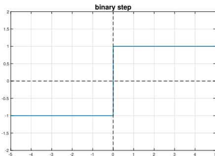
(a) Binary step activation function between -1 and +1 which was originally used in Hopfield networks
