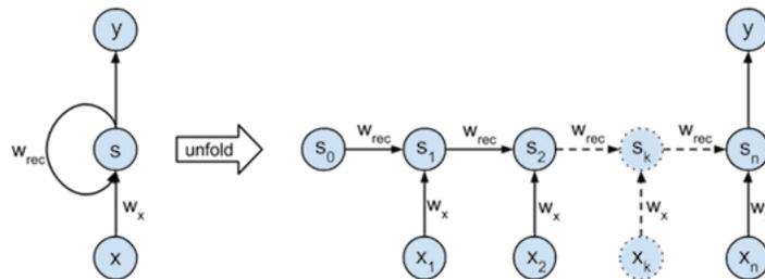
**Figure 2.12:** Unfolding of a recurrent layer into its feed-forward equivalent. Notice how the weights  $w_{rec}$  are shared across time and the input weight  $w_x$  is kept constant. The state of the network is updated at each time steps through the combination of the input and the recurrent contribution. Image was taken from [http://peterroelants.github.io/posts/rnn\\_implementation\\_part01/](http://peterroelants.github.io/posts/rnn_implementation_part01/)
