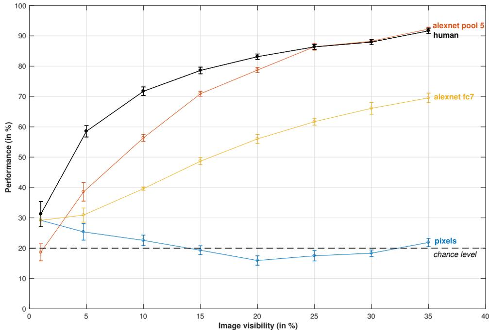
**Figure 4.5:** Performance of pool 5 (red) and fc7 (blue) layers of the feed-forward computational model named AlexNet. They can be contrasted to chance level (dashed line), raw pixel classification (blue) and human performance on the same dataset (black). Extracted features by Alexnet were classified using a SVM trained on whole objects and tested on partial renderings of the objects absent from the training set. Error bars are the s.e.m (5-fold cross validation).
