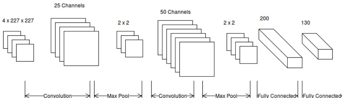
**Figure 2.9:** Example of a neural network architecture containing two convolutional layers, two pooling layers and two fully-connected layers. Image was taken from [https://filebox.ece.vt.edu/~aroma/web/cv\\_project\\_15/approach.html](https://filebox.ece.vt.edu/~aroma/web/cv_project_15/approach.html).
