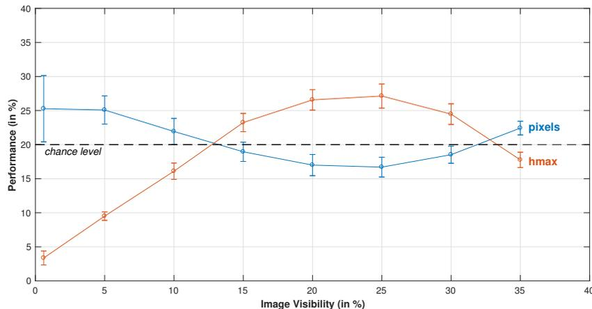
**Figure 4.4:** Performance of the HMAX computational model (red) compared to raw image pixels classification (blue). Chance level at 20% is represented by a dashed line. Extracted features by the HMAX model and pixel value were classified using a SVM trained on whole images and tested on occluded renderings. Occluded counterparts of objects used to train the classifier were not used in the test set. Error bars are the s.e.m across the 5 fold of cross validation.
