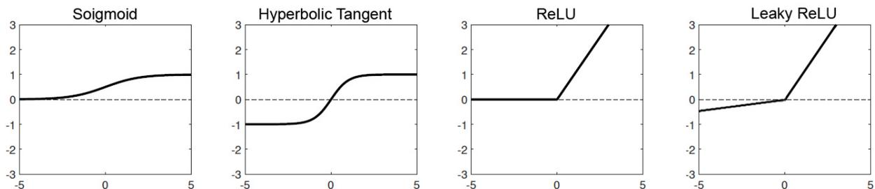
**Figure 2.8:** Different frequently used activation function. A common and necessary feature is non linearity. Sigmoid and hyperbolic tangent are saturating, increasing the problem of vanishing gradient while ReLU provides faster learning and sparser weights. Leaky ReLU is an attempt to minimize the risk of "dead" ReLU were the system is unable to update because of negative input and zero gradient.
