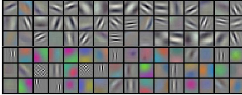
**Figure 2.10:** Examples of filters learnt by the first convolutional layer of Alexnet. Each of the 96 filters composing the convolutional layer is of size  $[11 \times 11 \times 3]$  for RGB images and each filter is shared by the  $55 \times 55$  neurons in one depth slice. Image was taken from the course <http://cs231n.stanford.edu/>
