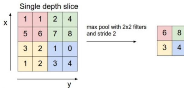
**Figure 2.11:** Example of a  $2 \times 2$  filter slid with a stride of 2 across the height and length of the activation map of a specific filter of a convolutional layer[43]. Image was take from the course <http://cs231n.stanford.edu/>
