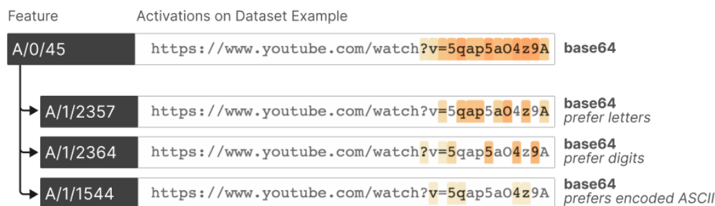
Figure 4.47: One base64 feature in the smaller dictionary with 512 features splits into three base64 features with the 4,096 feature dictionary.
